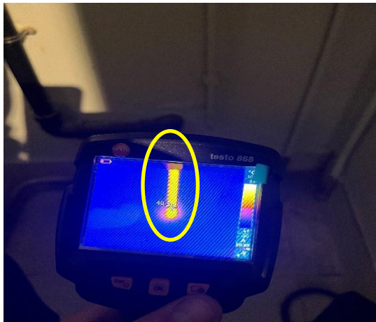
Pressure relief pipe hot under boiler
